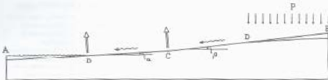
Fig. 1a: idealized section along a seepage face
